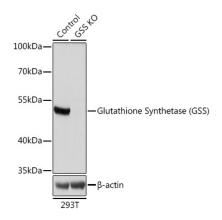
Western blot analysis of lysates from wild type (WT) and Glutathione Synthetase (Glutathione Synthetase (GSS)) knockout (KO) 293T cells, using [KO Validated] Glutathione Synthetase (GSS) Rabbit pAb (A14535) at 1:1000 dilution.
