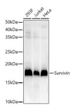
Western blot analysis of extracts of various cell lines, using Survivin antibody (A22034) at1:2000 dilution. Secondary antibody: HRP Goat Anti-Rabbit IgG (H+L) (AS014) at 1:10000 dilution.
