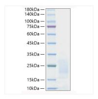
Recombinant Human Prostate stem cell antigen/PSCA Protein was determined by SDS-PAGE with Coomassie Blue, showing bands at 15-35 kDa.
