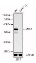
Western blot analysis of lysates from wild type(WT) and MEK7 knockout (KO) 293T(KO) cells, using [KO Validated] MEK7 Rabbit mAb (A12950) at 1:1000 dilution.
