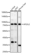
Western blot analysis of various lysates, using AFG3L2 Rabbit pAb (A23598) at 1:1000 dilution. Secondary antibody: HRP-conjugated Goat anti-Rabbit IgG (H+L) (AS014) at 1:10000 dilution. Lysates/proteins: 25µg per lane.
