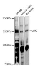
Western blot analysis of various lysates using APC Rabbit pAb (A2818) at 1:1000 dilution. Secondary antibody: HRP-conjugated Goat anti-Rabbit lgG (H+L) (AS014) at 1:10000 dilution. Lysates/proteins:  $25\mu g$  per lane.
