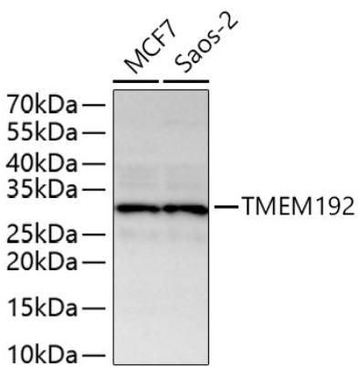
Western blot analysis of various lysates using TMEM192 Rabbit mAb (A28622) at 1:4000 dilution incubated overnight at 4°C.
