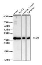
Western blot analysis of various lysates, using TFAM Rabbit pAb (A3173) at 1:1200 dilution. Secondary antibody: HRP Goat Anti-Rabbit IgG (H+L) (AS014) at 1:10000 dilution.
