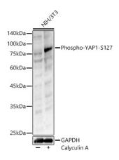
Western blot analysis of lysates from NIH/3T3 cells, using Phospho-YAP1-S127 Rabbit pAb (AP0489) at 1:400 dilution.NIH/3T3 cells were treated by Calyculin A (100 nM) at  $37^{\circ}\text{C}$  for 30 minutes after serum-starvation overnight.
