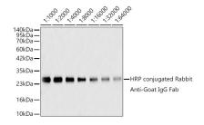
Western blot analysis of recombinant goat IgG Fab protein using HRP-conjugated Rabbit anti-Goat IgG Fab mAb(AS097) at 1:500-1:64000 dilution. Blot was incubated with the HRP conjugated antibody in the Blocking buffer (3% non-fat dry milk in TBST) at room temperature for 1 hour before detection using Enhanced chemiluminescence.
