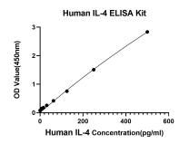
This standard curve is only for demonstration purposes. A standard curve should be generated for each assay.
