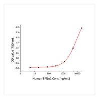
Immobilized Human EphA2 at 1  $\mu$ g/mL (100  $\mu$ L/well) can bind Human EFNA1 with a linear range of 4.883 ng/mL-9.206  $\mu$ g/mL.
