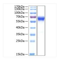
Recombinant Human TNFRSF9/4-1BB/CD137 Protein was determined by SDS-PAGE with Coomassie Blue, showing a band at 60-66 kDa.
