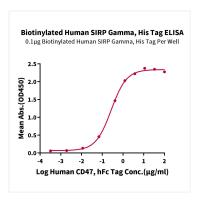
Immobilized Biotinylated Human SIRP Gamma, His Tag at 1  $\mu$ g/mL (100  $\mu$ L/well) on the streptavidin precoated plate (5  $\mu$ g/mL). Dose response curve for Human CD47, hFc Tag with the EC<sub>50</sub> of 0.27  $\mu$ g/mL determined by ELISA.
