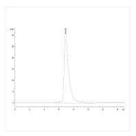
The purity of Biotinylated Human SIRP gamma is greater than 95% as determined by SEC-HPLC.
