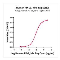
Immobilized Human PD-L1, mFc Tag at 2  $\mu$ g/mL (100  $\mu$ L/well) on the plate. Dose response curve for Human PD-1, hFc Tag with the EC<sub>50</sub> of 90.5ng/mL determined by ELISA (QC Test).
