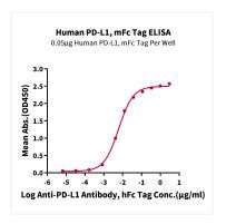
Immobilized Human PD-L1, mFc Tag at 0.5  $\mu$ g/mL (100  $\mu$ L/well) on the plate. Dose response curve for Anti-PD-L1 Antibody, hFc Tag with the EC<sub>50</sub> of 6.1ng/mL determined by ELISA.
