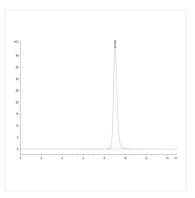
The purity of Human Fc gamma RIIIB (NA1) is greater than 95% as determined by SEC-HPLC.
