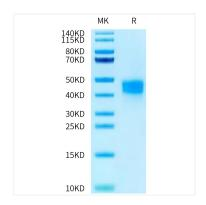
Human Fc gamma RIIIB (NA1) on Tris-Bis PAGE under reduced condition. The purity is greater than 95%.
