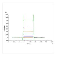
Human Fc gamma RIIIB (NA1), His Tag captured on CM5 Chip via anti-his antibody can bind Rituximab with an affinity constant of  $8.55~\mu\text{M}$  as determined in SPR assay (Biacore T200).
