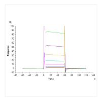
Biotinylated Human Fc gamma RIIB, His-Avi Tag captured on CM5 Chip via Anti-his antibody can bind Rituximab with an affinity constant of 5.87  $\mu$ M as determined in SPR assay (Biacore T200) (QC Test).
