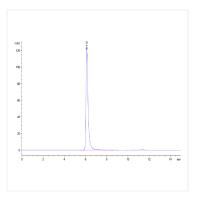
The purity of Human ALCAM is greater than 95% as determined by SEC-HPLC.
