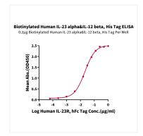
Immobilized Biotinylated Human IL-23 alpha&IL-12 beta, His Tag at 2  $\mu$ g/mL (100  $\mu$ L/well) on the streptavidin precoated plate (5  $\mu$ g/mL). Dose response curve for Human IL-23R, hFc Tag with the EC<sub>50</sub> of 21.0ng/mL determined by ELISA (QC Test).
