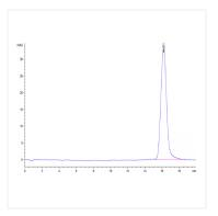
The purity of Biotinylated Human B7-H3 is greater than 95% as determined by SEC-HPLC.
