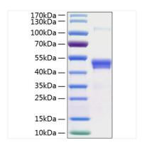
Recombinant Human TSG-14/PTX3 Protein was determined by SDS-PAGE with Coomassie Blue, showing a band at 45-50 kDa.
