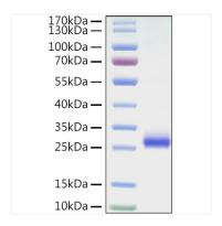
Recombinant Mouse TNFRSF5/CD40 Protein was determined by SDS-PAGE with Coomassie Blue, showing a band at 25-30kDa.
