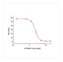
Recombinant Human TIMP-1 inhibit human MMP-2 cleavage of a fluorogenic peptide substrate Mca-PLGL-Dpa-AR-NH2. The IC50 value is approximately 2.2 nM.
