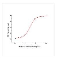
Immobilized Human IL10 (Catalog: RP00093) at 2  $\mu$ g/mL (100  $\mu$ L/well) can bind Human IL10RA (Catalog: RP01648) with a linear range of 0.1-2.9 ng/mL.
