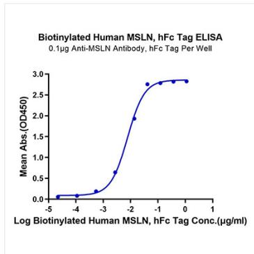
Immobilized Anti-MSLN Antibody, hFc Tag at 1 $\mu$ g/ml (100 $\mu$ l/well) on the plate. Dose response curve for Biotinylated Human MSLN, hFc Tag with the EC<sub>50</sub> of 7.7ng/ml determined by ELISA.
