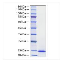
Recombinant Mouse Midkine Protein was determined by SDS-PAGE with Coomassie Blue, showing a band at 10-15 kD.
