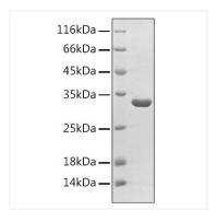
Recombinant Human PPAR-alpha//NR1C1 Protein was determined by SDS-PAGE with Coomassie Blue, showing a band at 25-35 kDa.
