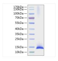
Recombinant Human CXCL17/VCC1 Protein was determined by SDS-PAGE with Coomassie Blue, showing a band at 12-18 kDa.
