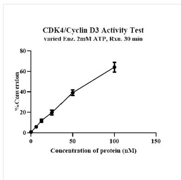
The activity of CDK4/Cyclin D3 is based on the MSA technology, and the content and ratio of the substrate and the product are directly separated and detected in real time and dynamically by the different migration rates of the substrate and the product after the enzymatic reaction.
