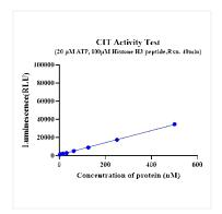
The activity of CIT is based on the ADP-Glo technology, and the ADP-GLO kinase activity assay quantifies kinase activity by measuring the conversion of ATP to ADP catalyzed by the kinase. Specific reagents are used to convert the ADP in the reaction back to ATP, resulting in the production of a luminescent signal.
